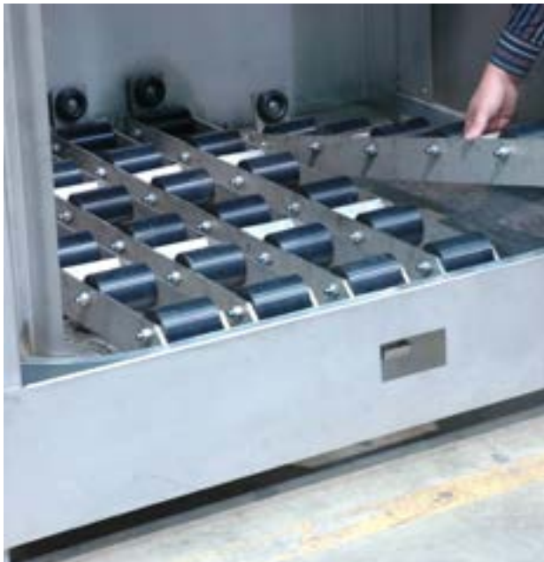
ABM - removable stainless steel roller strips
