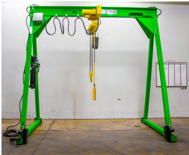
Gantry crane full front view with hoist
