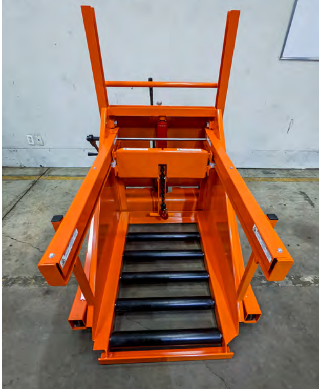
Convenient waist-high lifting and lowering using hand controls
