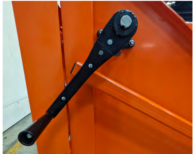
Crank handle to maneuver forklift battery into manual tugger
