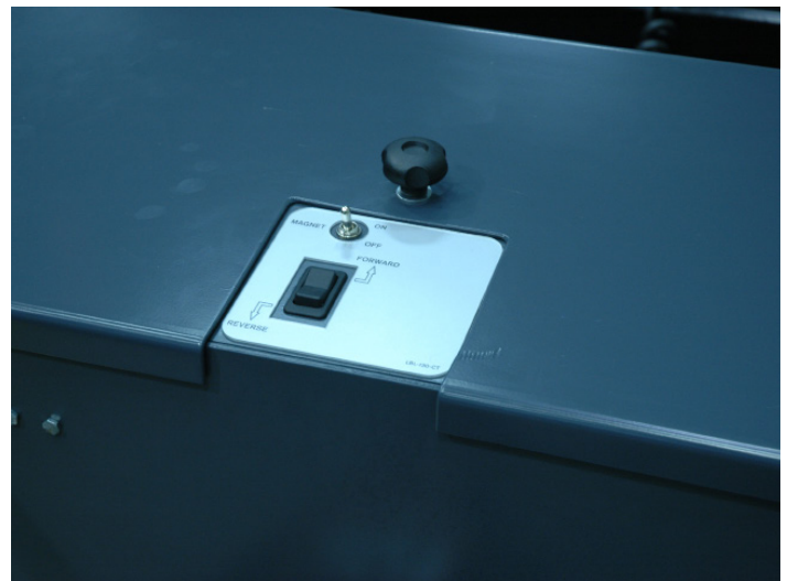
On/off switch for the battery extractor & forward/reverse switch
