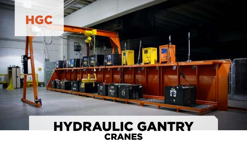
Despite the increased use of rollout battery extraction, there is still a need for safe, reliable, and effective lift-out gantry systems to support legacy and specialized equipment. CBH offers a range of gantry cranes in both fixed and mobile configurations, with manual and hydraulic drive options. Our unique hydraulic drive system utilizes positive traction on both sides to reduce twisting and frame stress, requiring only a floor guide on one side for better workspace utilization.
