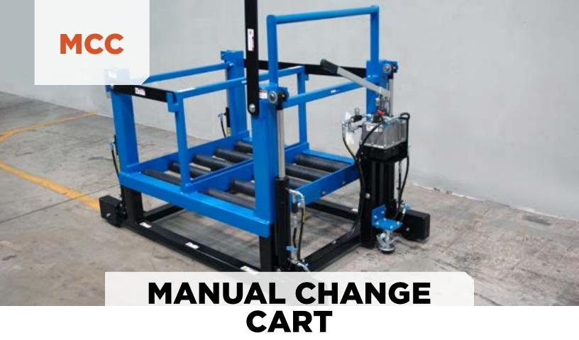
If your operation includes a small fleet of pallet trucks and order picker batteries, a manual extractor remains a low-cost, yet effective solution. Engineered to allow safe and effective manual battery changes with minimal effort, the MCC operates within its guide channels. The operator benefits from integrated battery stops, foot braking and loading and unloading from both sides of the system.
